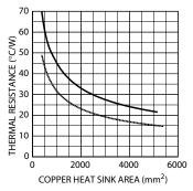
Figure 6. PCB Heat Sink Thermal Resistance
