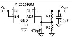
Figure 4. Ultra-Low-Noise Adjustable Application.
